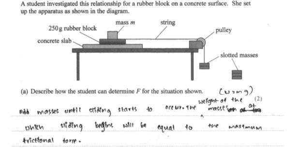
This response clearly describes adding slotted masses until the rubber block starts to slide and correctly describes how the force is then calculated, so scores 2 marks.
