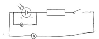
This example clearly shows an ammeter in series with the solar cell and a voltmeter in parallel with the solar cell so scores 2 marks.
